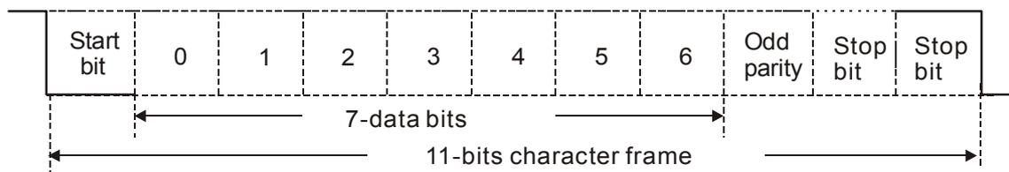
11-bit 字符框 (For RTU)
